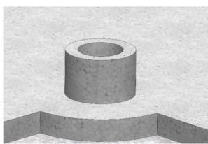
Instead of the floor box, it is first fitted with a polystyrene insert or formwork. The floor box has holes for cables: 2x from below / bottom and 2x from the side. The dimensions of the formwork should be approx. Ø152 mm x height 100 mm
