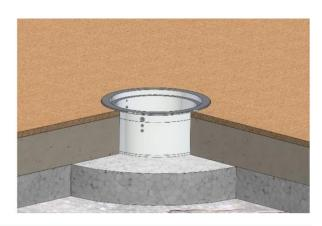
The floor box is installed from above. Insert the tube(s) with the cable(s) (or the cable itself) into the designated 25 mm holes. The enclosed Ø25 plugs are used to seal
