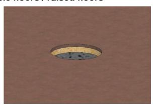
A hole of approx. Ø152 mm is drilled in the required place of the floor.
