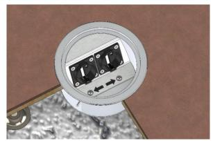
The floor box is fastened with the help of three side (inner) screws, or a mounting glue can be used (from the bottom of the upper frame / collar). Then connect the prepared cables to the sockets and fasten the socket holder back to the bottom of the floor box with two screws.
