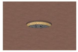
A hole of approx. Ø152 mm is drilled in the required place of the floor.
