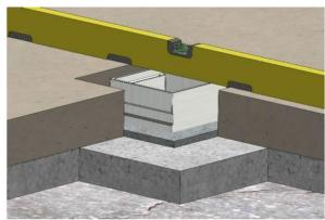
Insert pipe/s with wires into set holes (25mm). Attached end caps Ø25 are for unused hole. This end caps can be used as bushing (need to drill holes into it) for specific wires, it's possible to take out socket holder (including sockets) to prevent any damage during install. Floor box is pushed by water level into mortar/glue basis. Upper edge of the box should be levelled with concrete
