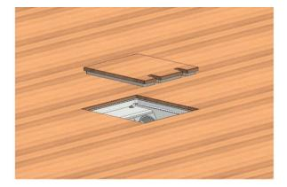
Cut the lid from floor material (Be careful about wood patterns!), size 125x125mm or depends on size of the hole made for the box. Glue aluminium lid (115x115mm) to the lid from floor material; be sure it's glued in the centre. Cut openings in relevant places for electric cords. If multiple holes not needed, you don't have to cut them out)
