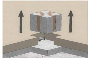
Place for floor socket/ First set up box, made from polystyrene or formwork (size should be 2-4 cm bigger than corresponding box for floor socket. After pouring concrete, remove polystyrene.
