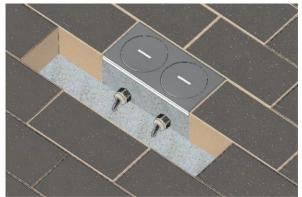
The floor box is placed in a prepared place so that it is possible to add paving (according to the shape and size of the paving). A mortar / concrete bed is prepared under the floor box and the entire floor box is fixed with concrete. Note: the floorer chooses the method of fixing / concreting the floor box (eg according to the type and height of the paving). Therefore, the installation may differ from this installation design.
