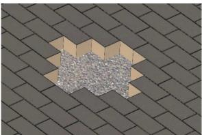
The paving is placed on the whole surface and then a part of the paving is removed (at the marked place).
