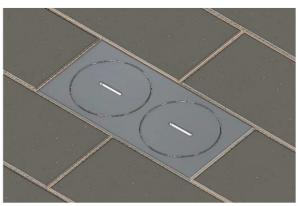
Before the concrete hardens, the floor box is leveled with the ground using a spirit level. Subsequently, the missing tiles will be added.
