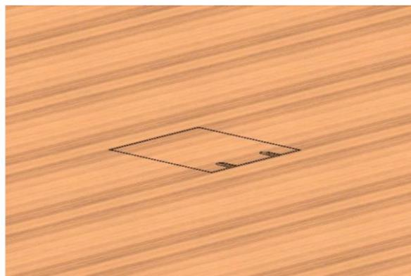
**4 spacing screws, which are always located in the corner of the box, allow for a slight (approx. 5 mm) adjustment of the lid height (lid lifting) so that the lid is in the same plane as the floor covering around the floor box.**
