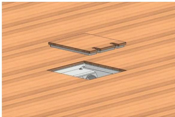
Cut the lid from floor material (Be careful about wood patterns!), size 240x240mm or depends on size of the hole made for the box. Glue aluminium lid (235x235mm) to the lid from floor material; be sure it's glued in the centre. Cut openings in relevant places for electric cords. If multiple holes not needed, you don't have to cut them out)
